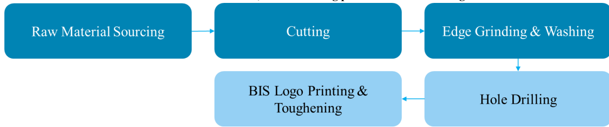
Exhibit 5.7: Process flow, manufacturing process for MWO bare glass
